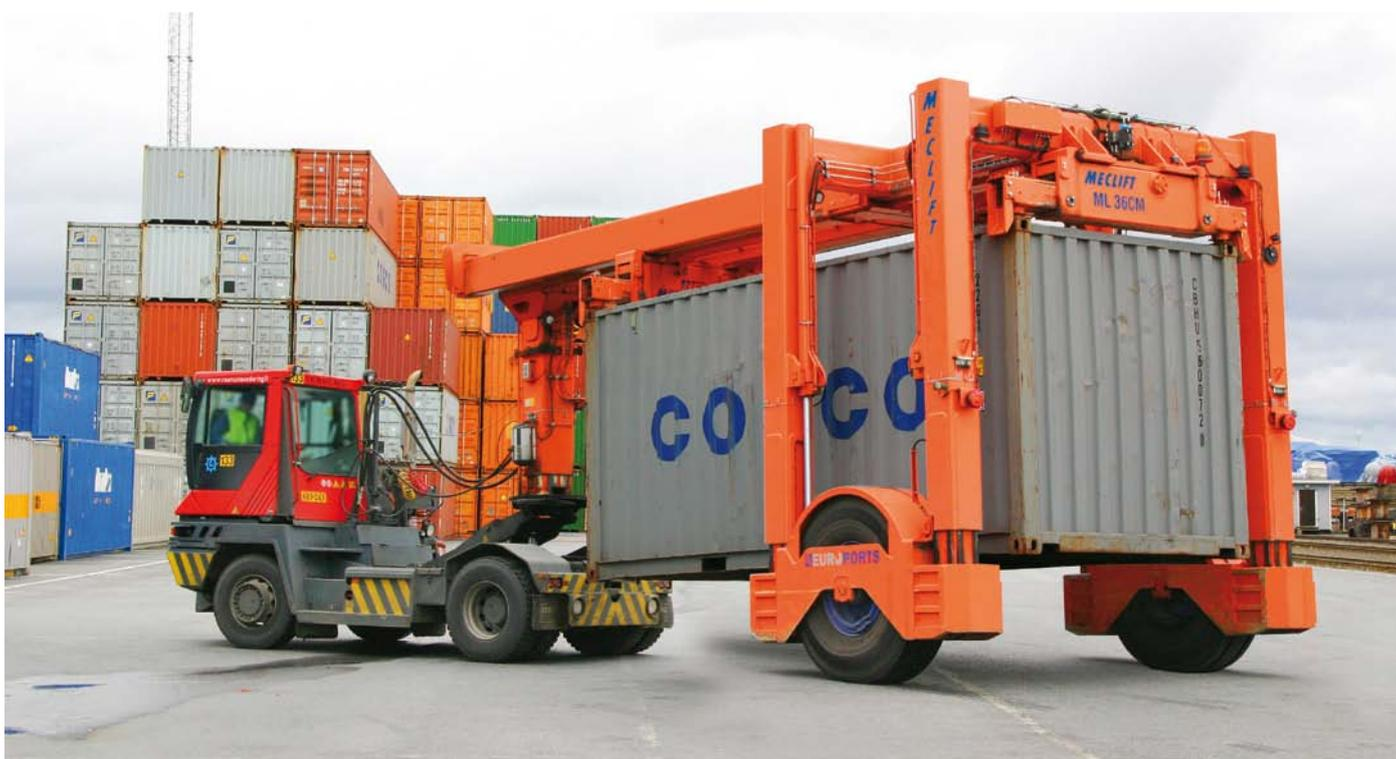
**The efficiency of the Meclift Container Mover ML36CM is proven daily at the Rauma Stevedoring port. The costs in horizontal container moving are only a half of similar operation by means of a reach stacker. In addition, longer transportations can be done with ML36CM only, without any other machinery. Improved work safety and ergonomics enhance smooth operation. Certain technical requirements taken into consideration, the machine can be attached to any terminal tractor.**
