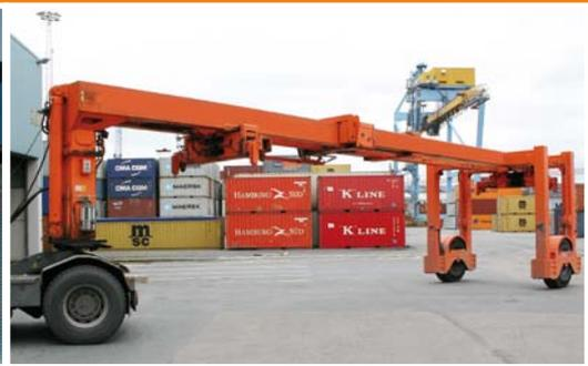
The length of the main beam is automatically adjustable for varying container sizes.
