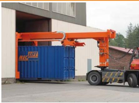
Compact design enables operating through terminal door openings.
